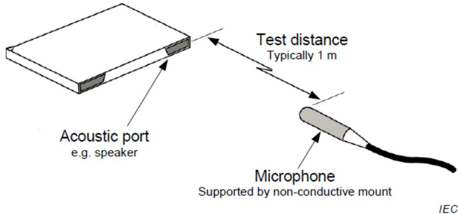
The microphone is connected via the cable to a suitable amplifier. Ensure that there is minimal acoustic loss between EUT and microphone.
