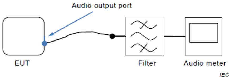
The filter is the audio filter specified in G.6.1 and is typically incorporated into the audio meter. Additional filtering might be necessary to ensure that the RF disturbance signal does not interfere with the measurement.
